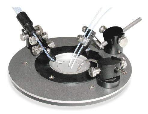
The perfusion manifolds are used to switch between multiple solutions during bath perfusion. This item is included with computerized perfusion systems. The manifold comes with short pieces of PTFE tubing, which fits to polyethylene tubing included with perfusion systems. These pieces can be easily replaced with different tubing of your choice. Use ferrule and luer-type fitting from PS-KIT to attach the manifold to different tubing, including 1/16" and larger I.D. soft tubing.
