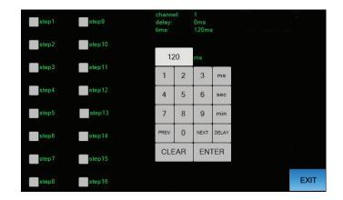
The touch pad on the right is used to enter time values in ms, sec or min. To switch between time and delay, touch "Delay"/"Time" button. To edit the values, use "Clear" button. Touch button "Enter" to put the new value into the controller memory. In order to mover between different channels values, touch buttons NEXT/PREV.
