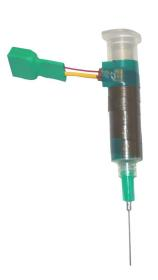
3. Make a loop using provided Velcro tape, and tighten it around the heater so the connector is sticking outside from the tape. Wrap the remaining Velcro tape around the syringe to prevent heat dissipation. You can use two Velcro tapes on both ends of the heater.
