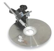
The manifold's metal body, a 4 mm O.D. stainless steel, can be mounted on miniature manipulators. The 4 mm rod can be also used to attach the manifold to magnetic holder MTH for small chamber perfusion. The included 7 mm adapter allows you to attach the manifold to regular size manipulators as well.
